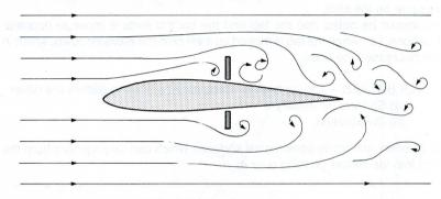
They are of robust construction and on some gliders may be used to limit the diving speed of a glider to a safe maximum. They are also used in the same way as spoilers to assist in controlling the approach. Their effects are:
