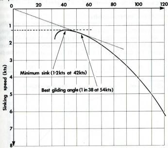
This graph gives a measure of the "penetration" of the aircraft which is the ability to increase its airspeed without an undue increase in sink. Thus at 42 knots the sink rate is 1.2 kt. and at 70 kt., 2.15 kt.; this corresponds to fairly good penetration.
