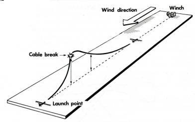
If space is limited, then a 'dog-leg' is the next possibility. A turn is made to one side, (usually the downwind side if there is any cross wind) through not more than 90°, and then back in the opposite direction. In the crosswind case the landing will then be more or less into wind.
