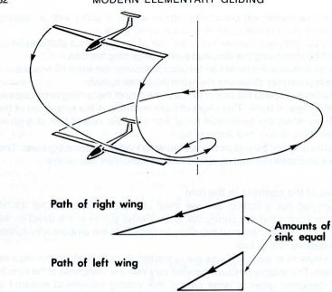
position. However, it is not necessary to think of the position of the stick; merely use the ailerons as necessary to keep the bank constant.
