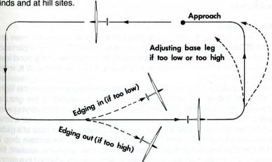
In a perfect circuit, the final turn into wind is made as the glider approaches the line of the landing run; however, the pilot can turn in and land at any time on the crosswind leg if he thinks that he is low. If the circuit has been made too high, height may be lost by the use of the airbrakes for a time on the base leg.
