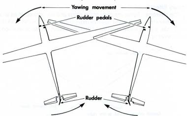
When the rudder pedal is pushed forward by the right foot, the rudder moves out to the right-hand side, and therefore is reacted on by the airflow. As a result
