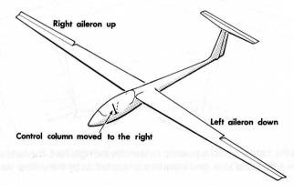
Movement of the stick to the left raises the left aileron and depresses the right aileron. Thus the left aileron presents a reduced angle of attack to the airflow, and therefore gives less lift; the right aileron, having been lowered, presents an increased angle of attack and hence gives more lift.
