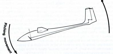
This pitching movement in flight alters the angle of attack of the wings to the airflow, and the balance of forces is upset, causing the flight path to change.
