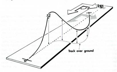
A circuit should only be attempted if the pilot is quite sure that he has ample height. If the straight-ahead or dog-leg options are not possible the likelyhood is that there is sufficient height for a circle or circuit, although any circuit is likely to be smaller than a normal circuit (see 44).
