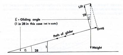
selects a speed not an angle of attack. The gliding angle is usually expressed as a ratio, e.g., 1 in 30. It should be noted that in the example above the angles are exaggerated for the sake of clarity (and, therefore the ratio of the forces is not representative).
