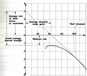
the glider flies between thermals. For this typical glider in England, a betweenthermal speed of 60 - 70 kt. according to the conditions is normally quite good enough.
