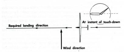
This counteracts any strain the touch-down might cause the undercarriage, by swinging the aircraft in line with the direction of motion; if this is done at the correct moment, the aircraft will touch down before the flight path has altered.
