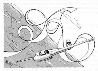
Before we go on to consider the effect of the controls is it essential to note this point: we will describe the action of the controls on the aircraft without any reference to the horizon, or any point on the earth. The controls always have the same primary effect relative to the aircraft (unless it is stalled) no matter what its position may be relative to the earth.
