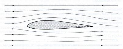
The result is that the air passing under the aerofoil increases in pressure and exerts an upward force on it, while the pressure of air passing over the top of the aerofoil is reduced and this exerts an upwards 'sucking' effect. These changes in pressure are actually quite small but both the air passing over and the air passing under have a lifting action.
