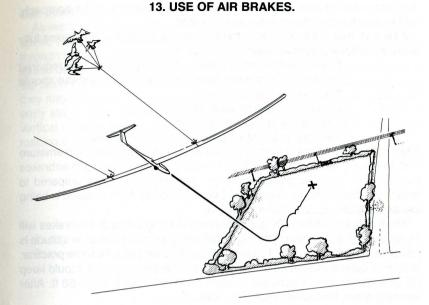
The air brakes fitted to gliders are of two alternative types, either spoilers or airbrakes. (Refer to page 23 for a description.) These are both used in the same way as an aid to landing, although the airbrakes are much more effective.
