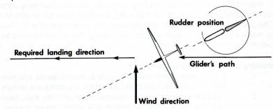
just before touching down, rudder should be applied in the direction of drift:-
