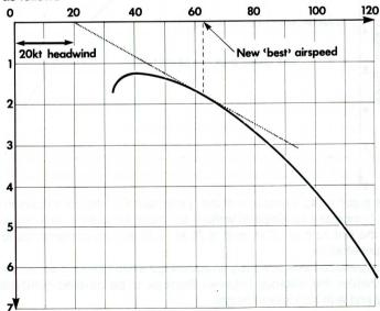
Along the airspeed axis lay off the amount of the headwind component; from this point reached, draw a new tangent to the polar curve; the point where it touched the curve corresponds to the "best" airspeed for those conditions.
