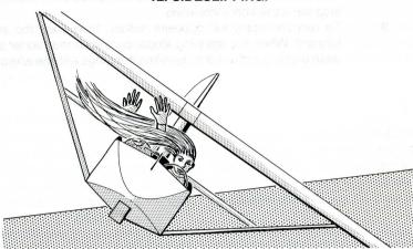
During a sideslip the aircraft is made to travel through the air partly broadside on, so that the line of flight is at an angle to the heading of the nose. This results in inefficient performance; the angle and rate of descent are increased without a corresponding increase in airspeed.
