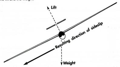
The steeper the angle of bank, the greater will be the sideways component of the motion. However, the sideslip is an unnatural condition of flight, with both
