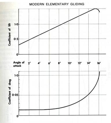
In order to make simple calculations using the lift and drag formulae, the correct values of the coefficients can be extracted from the above graphs.
