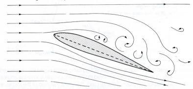
It is when the air over the aerofoil is in this turbulent state that the aerofoil is said to be stalled. Stalling occurs when the angle of attack is increased beyond the "stalling angle". The value of this angle depends on the design of the particular aerofoil. Stalling always occurs when the angle of the aerofoil relative to the airflow is increased beyond this value, and it cannot occur unless the angle is reached. Let us consider a set of circumstances in which the aircraft is stalled.
