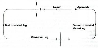
During the whole of the circuit, the pilot should be considering his position relative to the landing point, and making such adjustments to his direction of flight as he considers necessary. In the early stages of training, the landing point chosen should be some distance into the field to allow a margin for error.
