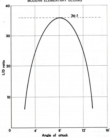
It was shown on page 13 that the angle of glide (in still air) is flattest when the ratio L/D is a maximum. Observe that this occurs at an angle of attack of about 7°; at normal loading this corresponds to an airspeed of about 50 Knots.
