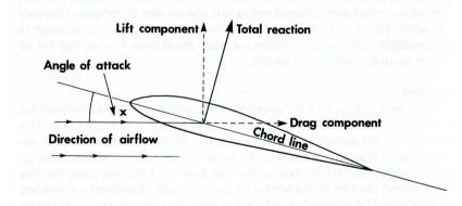
In the diagram here we represent each force by a line in the direction in which the force is working. The length of the line represents the strength of the force involved.
