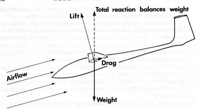
Similarly the lift of the aerofoil is obtained from all over the wing, but the total effect can be represented as one force passing through the Centre of Pressure. The Centre of Pressure bears the same relationship to lift as the centre of gravity does to weight but while the Centre of Gravity remains fixed, the centre of pressure's position varies depending on the angle of attack and the distribution of lift over the wing.
