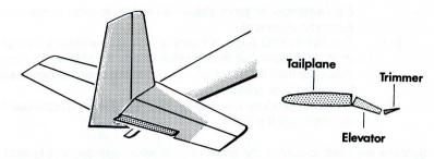
The trimmer is used to relieve the pilot of work in maintaining the required attitude in pitch. If, for instance, the pilot wishes to fly faster, he moves the stick to effect the necessary change of attitude and then, once the speed is steady, adjusts the trim until the aircraft maintains that attitude without any need for pressure on the stick.
